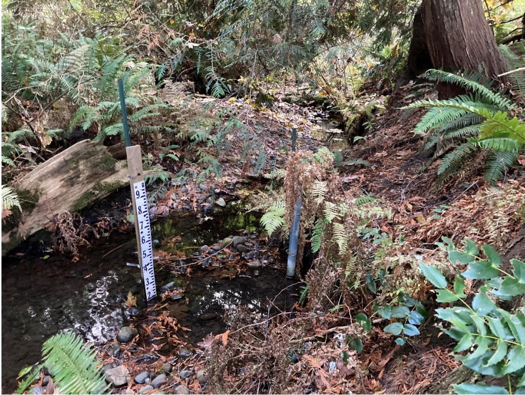
Figure 2. Photo depicts level logger and staff gauge location in Shelly Creek. 2022.
