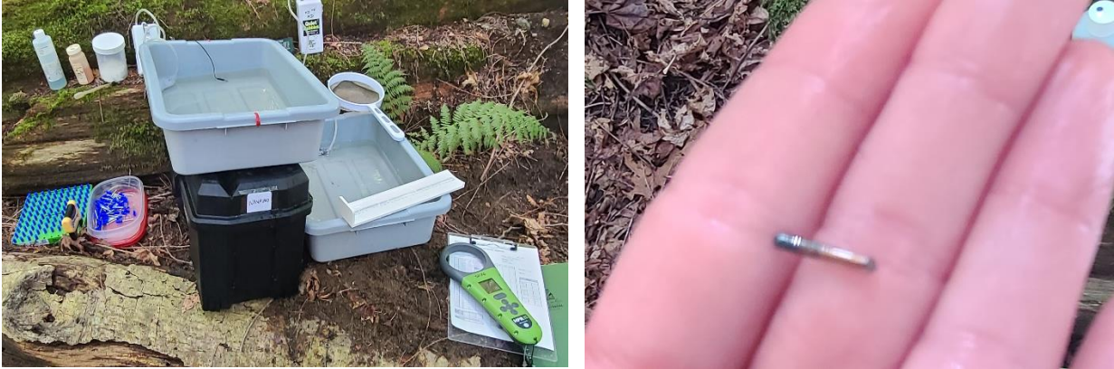
Figure 3. The left image PIT-tagging kit shows the HPR scanner, MK25 tagging gun, pre-loaded FDX-B tagging tray and static baths with MS222 and aerators. The right image shows the 12 mm FDX-B PIT tag.
