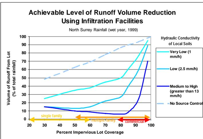
Where soils have medium or better hydraulic conductivity, runoff volume could be reduced to about 10% of total rainfall for all but the highest coverage land uses.
