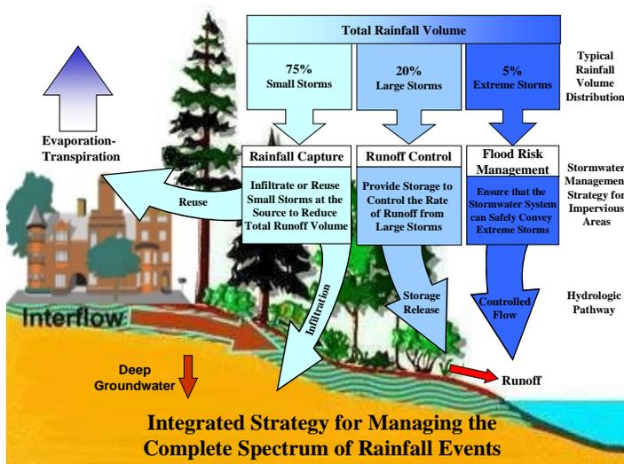
The WBM enables modelling of all three components of the Integrated Strategy for managing the complete rainfall spectrum – that is, *retain* the small frequent events, *detain* the large events, and *convey* the extreme events.
