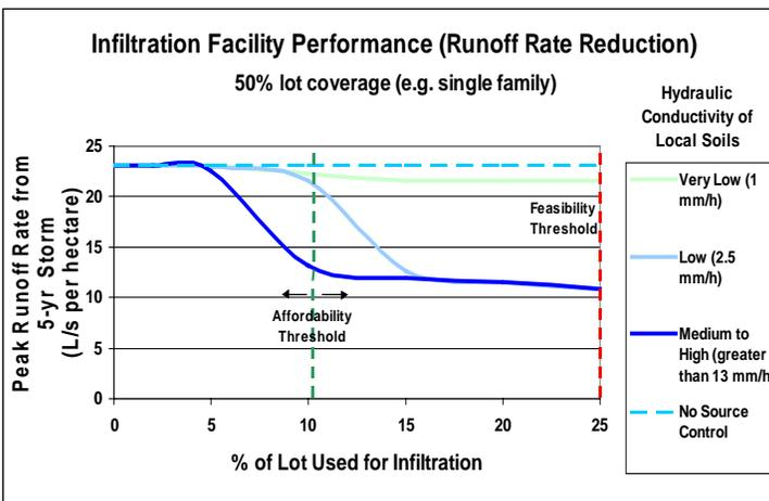
Reductions in runoff rates using infiltration facilities depend on the hydraulic conductivity of local soils and the amount of area provided for infiltration.
