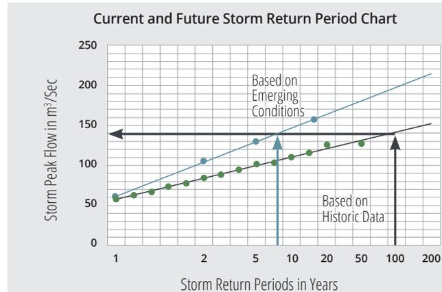
Figure 2. Historic and emerging stormflow return period due to increased climatic variability and increased impervious surfaces. The historic line formed the basis for designing stormwater and flood protection infrastructure (In this example a 100 year historic storm would now likely occur every 7 years - based on blue line).
