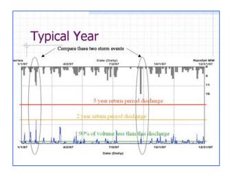
This hydrograph for a 'typical year' illustrate the variable response of a watershed to rainfall. Two events are highlighted in the graphic. The larger of the two rainfall events resulted in much less runoff. As can be seen from the hydrograph, the smaller of the two rainfall events was preceded by a period of wet weather such that more runoff resulted.
