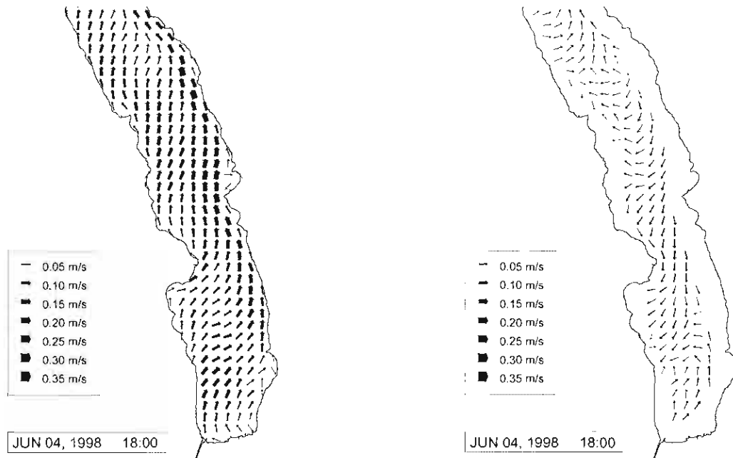
Figure 8. Velocity Flow Field on June 4, 1998 18:00. Left hand panel: at surface layer. Right hand panel: at depth of 28 m.
